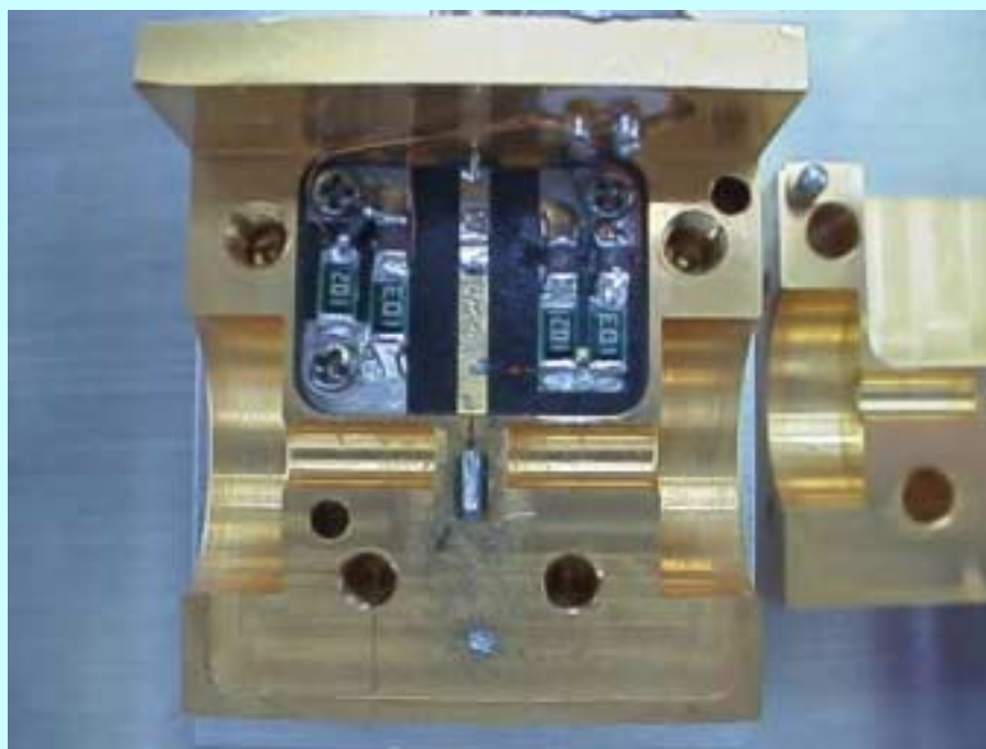
Inside of 640-GHz SIS mixer. DC-bias circuit is shown.
